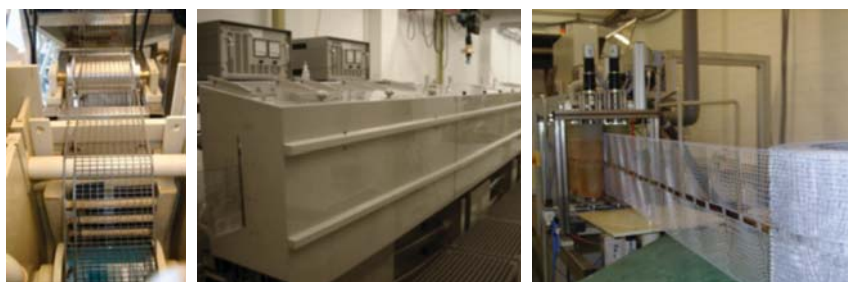
Figure 2: Production equipment for composite grids. Left: strip galvanofforming unit (open, without electrolyte); centre and right: multi-layer strip forming line consisting of a number of independent galvanic strip coating modules
